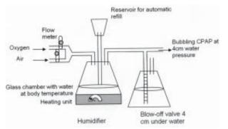
FIG. 1. Circuit for bubbling CPAP with blow-off valve 4 cm under water and autoclavable-glass humidifier unit.
